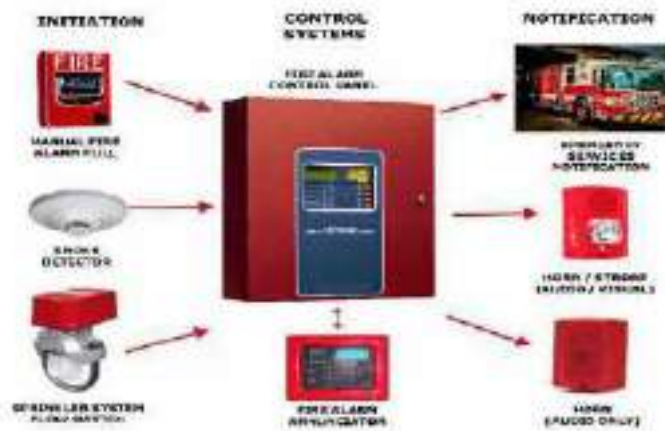
Addressable Main Fire Alarm Control Panel (FACP)
